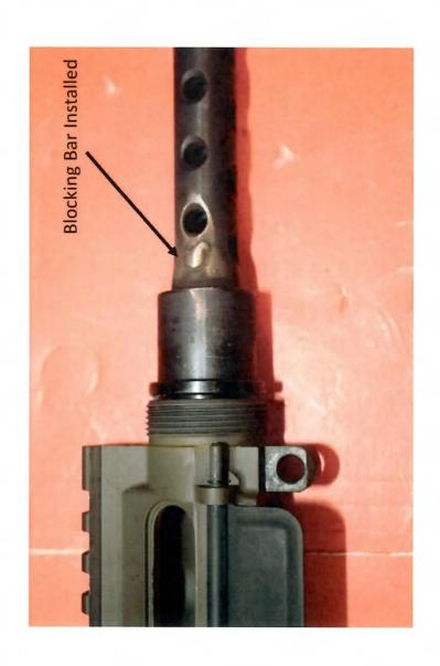
Blocking Bar Welded In Front of Chamber
