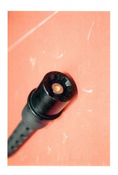
Front of "Barrel Portion" Welded to Prevent Projectile From Exiting
